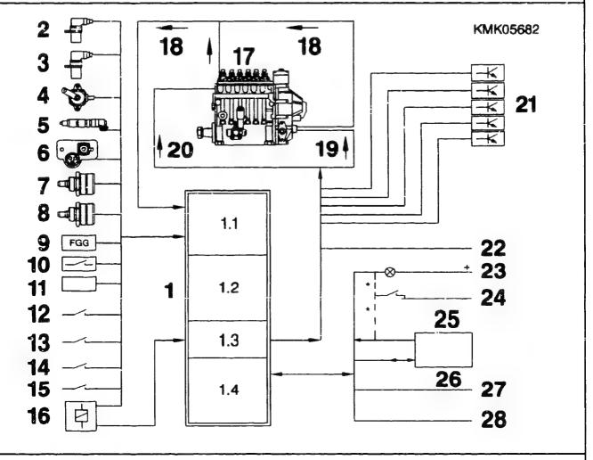
To regulate the injected quantity, an RPS (half-differential inductive pick-up) installed in the RE positioner constantly determines the instantaneous CRT and supplies the values (U/actual value) to the control unit.
